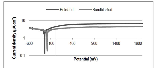
Fig. 3. Polarisation curves of plasma nitrided in 35:65 H<sub>2</sub>:N<sub>2</sub> gaseous mixture 440B steel in 0.9 wt% NaCl solution (unde-aerated, unstirred)
