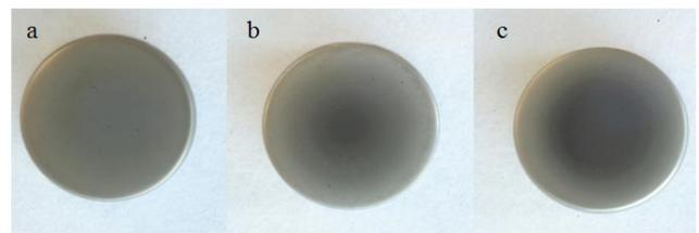
Fig. 7. Plasma nitrided polished specimens; a – 50% H<sub>2</sub>:50% N<sub>2</sub>, b – 35% H<sub>2</sub>:65% N<sub>2</sub>, c – 20% H<sub>2</sub>:80% N<sub>2</sub>; macro photographs
