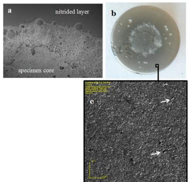
Fig. 8. Corroded surface morphology of plasma nitrided in 35:65 H<sub>2</sub>:N<sub>2</sub> working gas mixture 440B steel; a – SEM photograph, magnification 50×; b – macro photograph; c – confocal microscope photograph in 1080× magnification, arrows – transition phase particles
