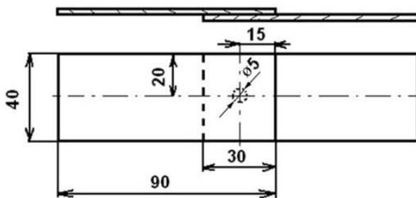
**Fig. 2.** Dimensions of the sample for tensile test
