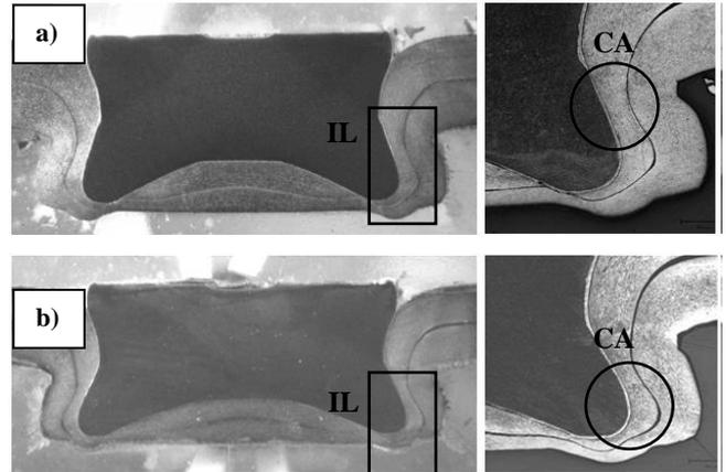
Fig. 7. ClinchRivet joints with interlocking and critical areas: a) H220PD, b) DX51D+Z (IL – interlocking, CA – critical area)
