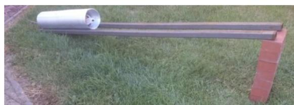
Fig. 14. The maximum pipeline slope test bench
