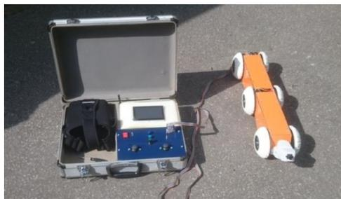
Fig. 16. The pipe inspection robot prototype and the control panel
