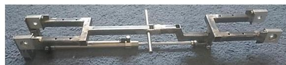
Fig. 8. The robot chassis basic configuration
