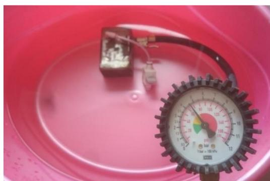
Fig. 10. The air pressure tank leak test
