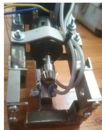
Fig. 9. The robot drive system
