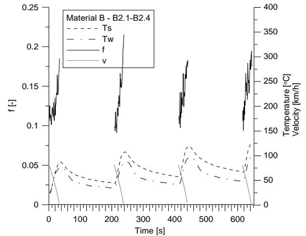
Fig. 8. Results of the second section of the full-scale dynamometer test – Material B
