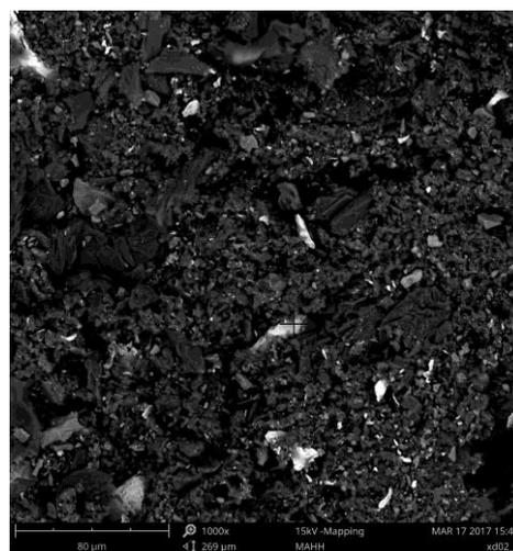
Fig. 2. Dispersion of the steel fibre (marked with a black cross) in the composite (Material B)
