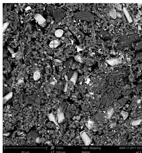
Fig. 1. Dispersion of the glass fibre (marked with a black cross) in the composite (Material A)
