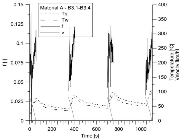
Fig. 6. Results of the third section of the full-scale dynamometer test – Material A
