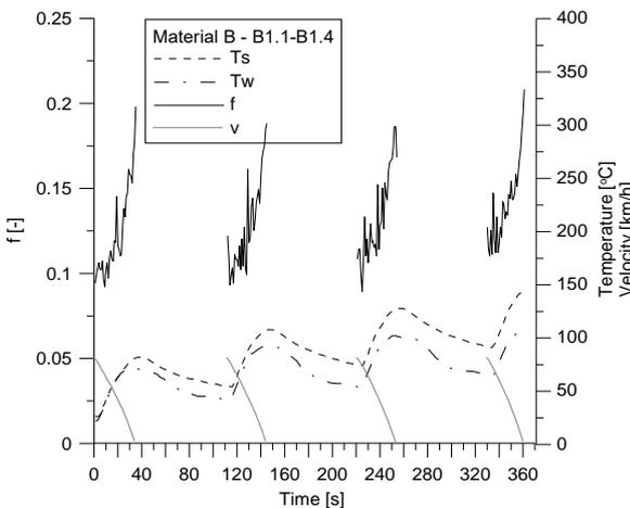
Fig. 7. Results of the first section of the full-scale dynamometer test – Material B
