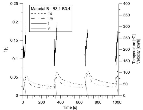
Fig. 9. Results of the third section of the full-scale dynamometer test – Material B
