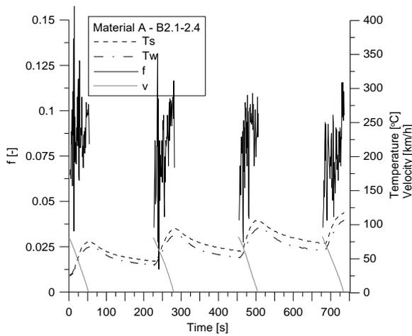
Fig. 5. Results of the second section of the full-scale dynamometer test – Material A
