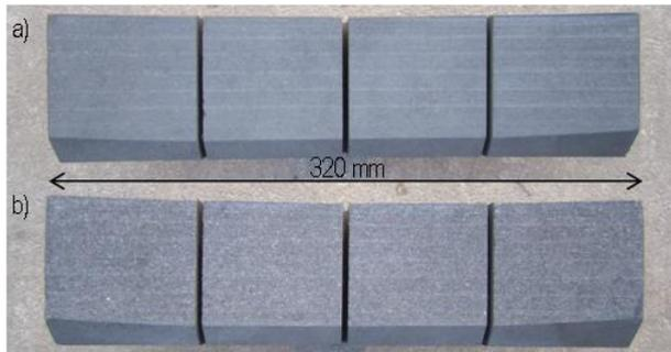
Fig. 3. View of the tested organic composite brake shoes: a) manufactured from Material A; b) manufactured from Material B
