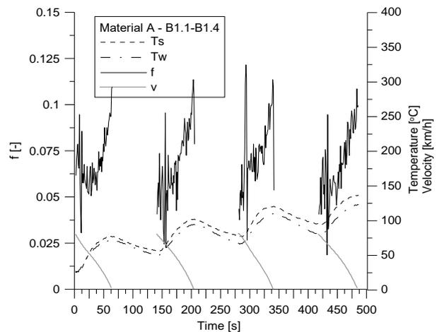
Fig. 4. Results of the first section of the full-scale dynamometer test – Material A
