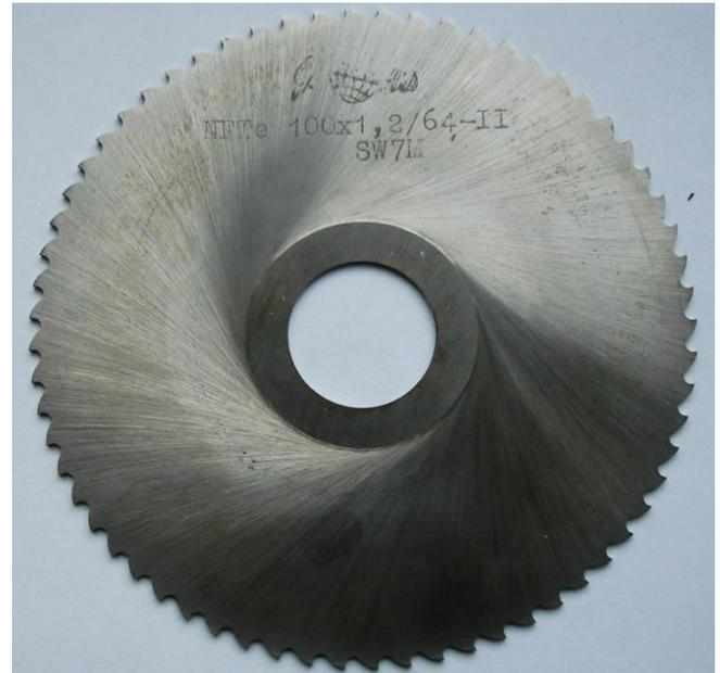
**Fig. 6.** NFTe 100x1.2/64-II circular slitting saw
