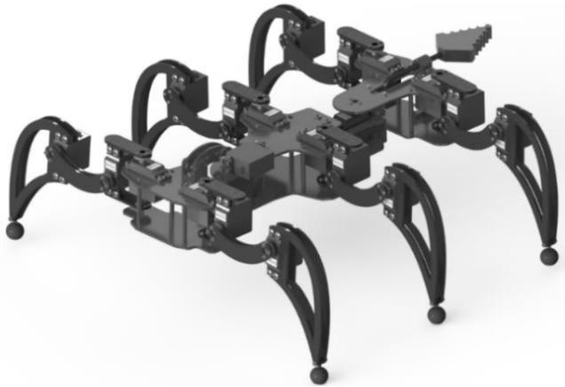
Fig. 2. 3D model of the hexa-quad bimorph walking robot in HEXAPOD configuration
