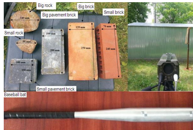
Fig. 3. Blunt objects and baseball bat used in the kinetic energy evaluation test with high-speed camera
