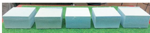
Fig. 6. Samples after the tests with a flat stamp
