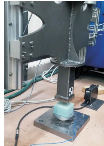
Fig. 2. A specimen placed on the support plate of the drop hammer with a flat beater installed on the beam
